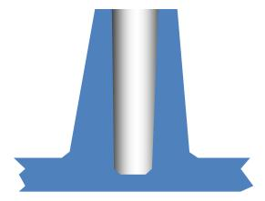
Whenever possible, bosses should not be directly connected to external walls. Instead, bosses should be connected to the walls using ribs.
