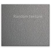
When applying a texture, it is important to remember that deeper textures may require steeper draft angles.
